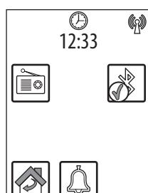
If there are no devices connected, in the top right corner the Bluetooth icon will appear barred and blinking.
